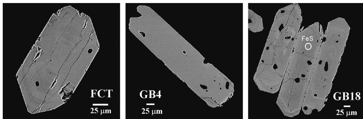
Fig. 1. Backscattered electron images taken on the WSU electron microprobe of zircons from Fish Canyon Tuff (FCT) and the Gold Butte granite at pre-exhumation paleodepths of 15 (GB4) and 4 km (GB18). The two large inclusions in the FCT zircon are alkali-feldspar with minor quartz. Subtle compositional zonation is indicated by the weak concentric shading zonation in FCT. Inclusions in the GB4 zircon are alkali-feldspar \pm quartz, except for the largest inclusion in the lower-right corner of the crystal, which is biotite. Inclusions in GB18 zircons are also dominantly alkali-feldspar \pm quartz; small inclusion labelled “py” in center grain is iron-sulfide. Weak concentric compositional zonation is apparent in these (but not all) GB18 zircons.
