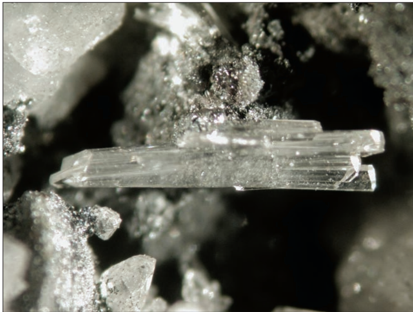
Figure 1. The largest cluster of crystals of stibioclaudeite, 6 mm across, in a vug of massive tennantite with quartz crystals. This is the holotype specimen. D. W. Bunk specimen, now in the W. W. Pinch collection.
