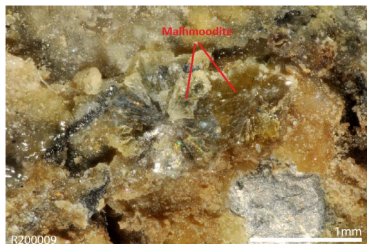
FIG. 2. A microscopic view of yellowish, flat-lying plates, divergent groups of malhmoodite crystals.
