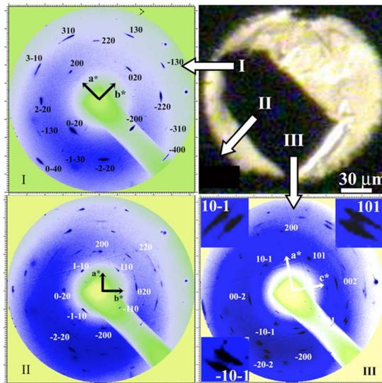
FIG. 2. (Color online) The images of a  $\text{Fe}_{1-x}\text{O}$  single-crystal in a diamond-anvil cell at 35 GPa and the corresponding observed diffraction patterns from Locations I, II, and III of the sample in a diamond-anvil cell. The indexing of each pattern has also been shown. The inserts in Patterns III are the enlarged splitting of diffraction class 101.
