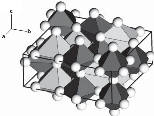
FIGURE 1. Structural image of karrooite ( $\text{MgTi}_2\text{O}_3$ ) that consists of two symmetrically distinct edge-sharing octahedral sites. When completely ordered, all Ti is located in the M2 site.
