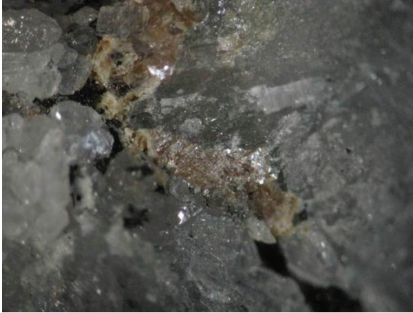
FIGURE 1. Pinkish-brown pauloabibite intergrown with an unidentified Ca-Nb oxide, with dolomite (white) and tochilinite (black), from the Jacupiranga mine, Cajati, São Paulo, Brazil. Field of view: 4 mm.
