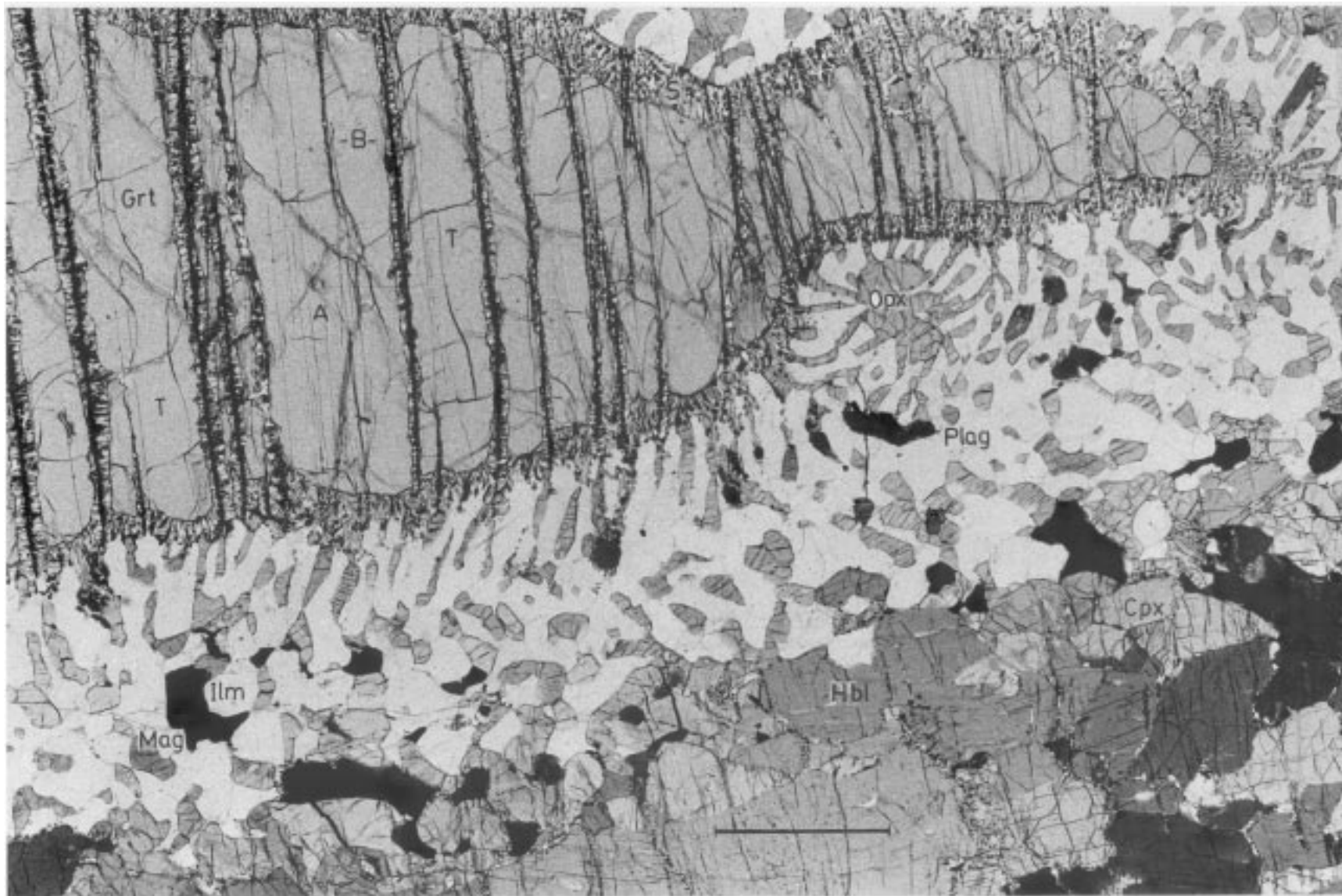
Figure 2. Photomicrograph showing the reaction texture and fracture cleavage of a large garnet grain in the sample 881307. The coarse grained outer symplectite, interpreted to have developed during the M1 decompression, consists of orthopyroxene (Opx) and plagioclase (Pl), with minor hornblende (Hbl) and magnetite (Mag)-ilmenite (Ilm) intergrowths. The finer grained inner (M2) symplectite mantling the grain and within the fracture zones consist of Opx, Plag and spinel (Spl) (+Mag-Ilm). Scale bar is 1.7 mm.
