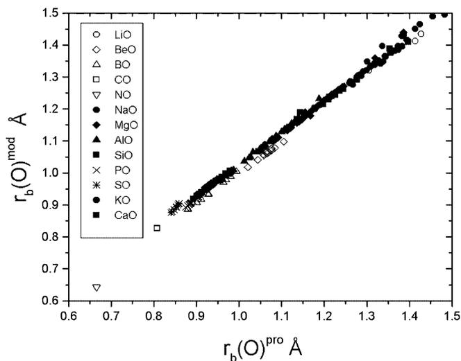
**Fig. 2** The bonded radius of the O atom determined from procrystal calculations,  $r_b(\text{O})^{\text{pro}}$ , versus that determined from ab initio model calculations,  $r_b(\text{O})^{\text{mod}}$ , for more than 300 MO bonds in minerals. The trend of the data demonstrates not only that the procrystal model reproduces all bond critical points found in the ab initio model calculations, but also the similarity in their locations
