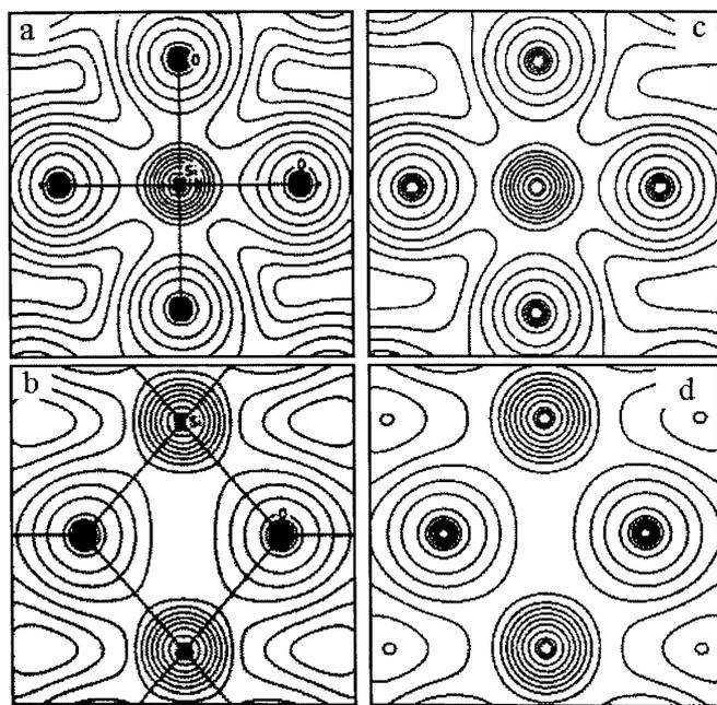
**Fig. 1a–d** Electron-density distributions (a and b) observed for stishovite (Spackman et al. 1987) are compared in c and d with those calculated for the corresponding procrystal distributions. Both were evaluated in the planes passing through the Si atom with a and c paralleling (111) and b and d paralleling (110). Despite the greater localization of the electron density displayed along the SiO bonds of the observed maps, the topography of the two distributions shows a close correspondence
