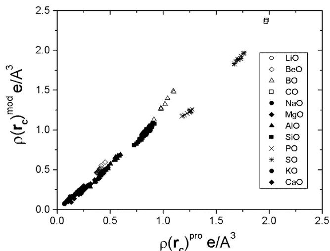
**Fig. 3** The magnitude of the electron density at the bond-critical point computed with the procrystal calculations,  $\rho(\mathbf{r}_C)^{\text{pro}}$ , compared to that computed with the ab initio model,  $\rho(\mathbf{r}_C)^{\text{mod}}$ . The data demonstrate that  $\rho(\mathbf{r}_C)^{\text{mod}}$  tends to be larger than  $\rho(\mathbf{r}_C)^{\text{pro}}$ , with a systematically increasing difference displayed by bonds with electronegative cations
