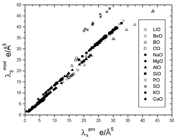
**Fig. 5** The curvatures of the electron density at the bond-critical point in the direction parallel to the bond are compared for the procrystal,  $\lambda_3^{\text{pro}}$ , and the ab initio model calculations,  $\lambda_3^{\text{mod}}$
