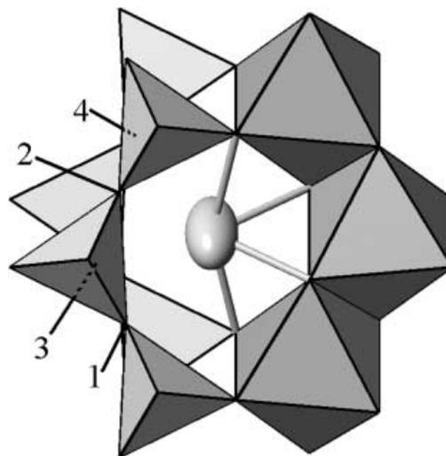
**Fig. 9** A portion of the structure of a pyroxene with  $SiO_4$  groups rendered as tetrahedra,  $M1O_6$  groups as octahedra, and the  $M2$  atom as a displacement ellipsoid. All O3 atoms bridge the tetrahedra, and are labeled to define the positions 1–4, as used in the text. The bonds between  $M2-O1$  and  $M2-O2$  are indicated by rigid rods
