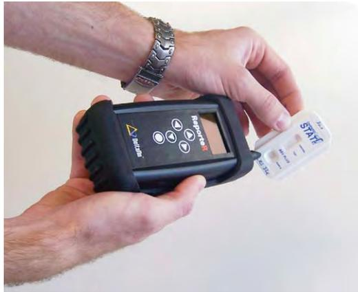
*The Reporte<sup>®</sup> system, an eleven ounce Raman spectrometer developed by DeltaNu. When released, it will be the first pocket-sized Raman system. As Raman technology continues to develop, it is anticipated that Raman spectrometers will become more portable for practical use by the public. Photo courtesy of DeltaNu, Inc.*
