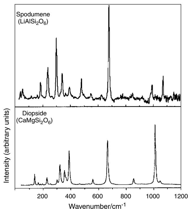
**Figure 6.** Top,  $C2/c$  spodumene on (110) face, and bottom,  $C2/c$  diopside on (110) face. Reference 19 assigns the vibrational regions in pyroxenes as follows: 800–1200  $\text{cm}^{-1}$  Si– $\text{O}_{\text{nb}}$  stretch, 650–800  $\text{cm}^{-1}$  Si– $\text{O}_{\text{b}}$  stretch, 425–650  $\text{cm}^{-1}$  Si–O bend and 50–425  $\text{cm}^{-1}$  complex lattice vibrations due to Si–O bend and M–O interactions.
