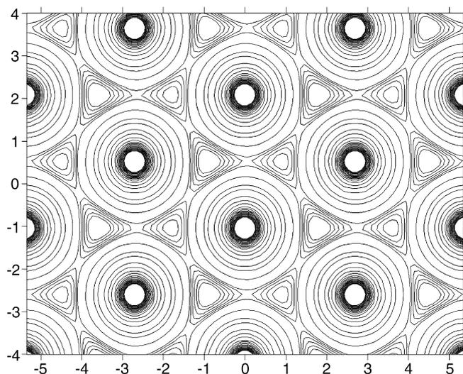
Fig. 2. A contour map of the procrystal electron density distribution through the plane with  $z = 0.25$  in  $\text{Ti}_3(\text{Si}_{0.43}\text{Ge}_{0.57})\text{C}_2$ . The contours presented are between 0 and  $10 \text{ e/\AA}^3$ . The unit of numbers on the horizontal and vertical axes is in Angstrom. Note the six bond paths around each Si/Ge atom. These bond paths indicate Si–Si bonds and may provide conduits for electron transfer.
