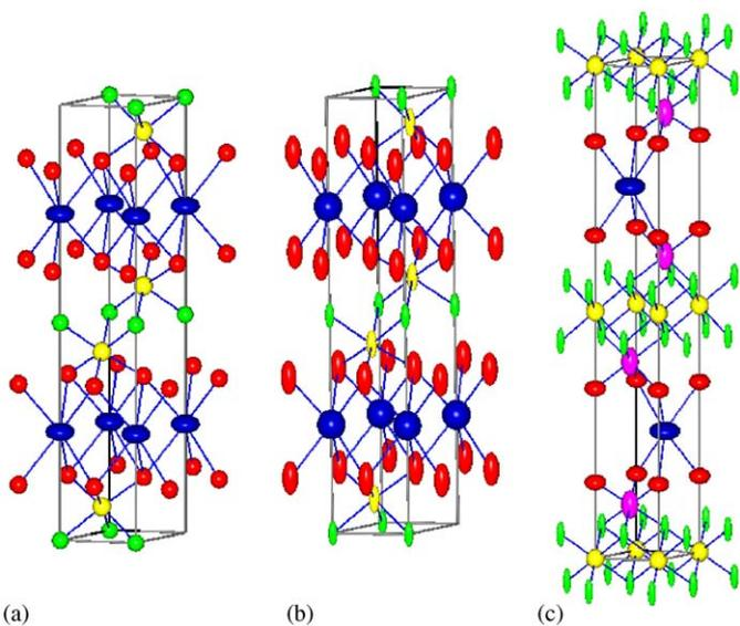
Fig. 1. Crystal structures of MAX phases: (a)  $\text{Ti}_3(\text{Si}_{0.43}\text{Ge}_{0.57})\text{C}_2$ , (b)  $\text{Ti}_3\text{SiC}_2$  [6], and (c),  $\text{Ti}_4\text{AlN}_3$  [7]. Thermal ellipsoids are drawn with 99% probability. In all figures, green and red ellipsoids represent Ti1 and Ti2 atoms, respectively, blue ellipsoids, (Si + Ge) or Al, and yellow and pink ellipsoids C or N.
