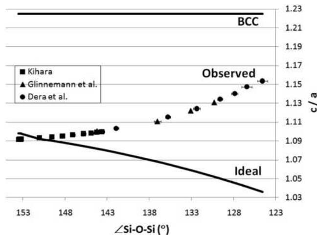
FIGURE 7. The  $c/a$  axial ratio vs. Si-O-Si angle for four structures: ideal quartz with perfectly regular tetrahedra, observed quartz (model quartz has the same ratio), and BCC quartz. All of the vertical error bars and some of the horizontal ones are too small to be seen.
