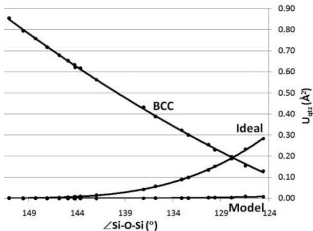
FIGURE 9. A comparison of three hypothetical structures with observed quartz.  $U_{\text{qtz}}$  is a measure of the similarity of one quartz structure to another. A value of 0 is an exact match (the structures are identical), while a value of 1 is a very poor fit. As Si-O-Si angle decreases, quartz is becoming more like BCC quartz and less ideal.
