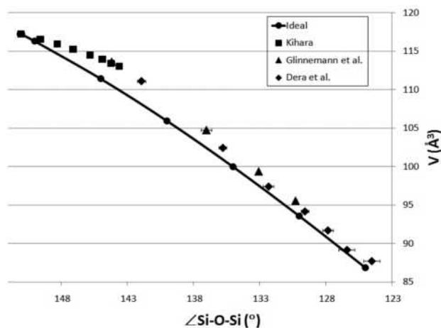
**FIGURE 1.** Volume vs. Si-O-Si angle in ideal and observed quartz. Ideal quartz has perfectly regular tetrahedra and in this figure is compressed by Si-O-Si angle-bending alone. Data from Kihara (1990), Glinnemann et al. (1992), and Dera et al. (in prep). Some horizontal and all vertical error bars too small to be seen.
