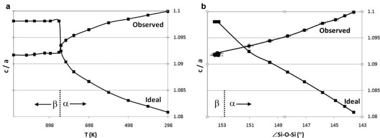
**FIGURE 5.** The  $c/a$  axial ratio for observed and ideal quartz plotted against (a) temperature and (b) Si-O-Si angle. This plot illustrates two points. First, that a parameter vs. temperature plot for  $\beta$ -quartz is often a horizontal line that collapses to a point in a parameter vs. angle plot. Second, that the  $c/a$  ratio for observed and ideal quartz is diverging as temperature decreases. All temperature error bars and some of the others are too small to be seen.
