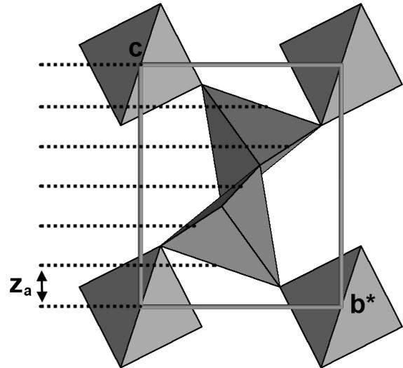
APPENDIX FIGURE 5. Deriving the  $c$  cell edge of ideal  $\alpha$ -quartz. Each dotted line passes through the midpoints of the edges of tetrahedra. Thus, the same vertical percentage of each tetrahedron is between dotted lines and  $c = 6z_a$ .
