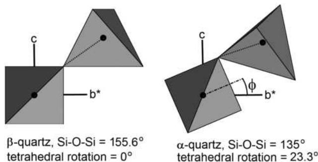
**FIGURE 6.** The relationship between the tetrahedral rotation angle,  $\phi$ , and the Si-O-Si angle,  $\theta$ . Ideal  $\beta$ -quartz has a rotation angle of 0° and an Si-O-Si angle of 155.6°. An ideal  $\alpha$ -quartz is also illustrated with a rotation angle of 23.3° and an Si-O-Si angle of 135°.
