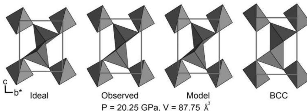
**FIGURE 4.** A comparison of observed quartz at 20.25 GPa (Dera et al. in prep) with three hypothetical structures with the same volume: ideal quartz, model quartz, and BCC quartz. Ideal quartz has regular tetrahedra and Si-O-Si angle equal to the observed, model quartz additionally has the same  $c/a$  axial ratio as observed.
