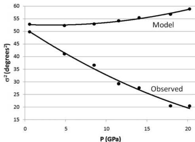
**FIGURE 11.** The similarity to the BCC tetrahedron in observed and model quartz. Intrafacial variance (Thompson and Downs 2010) is a cation-independent measure of the fit between a tetrahedron and the BCC Sommerville tetrahedron (O’Keeffe and Hyde 1996). The Si-tetrahedron in observed quartz is becoming more like the BCC tetrahedron as pressure increases, while the tetrahedron in model quartz is diverging from BCC.
