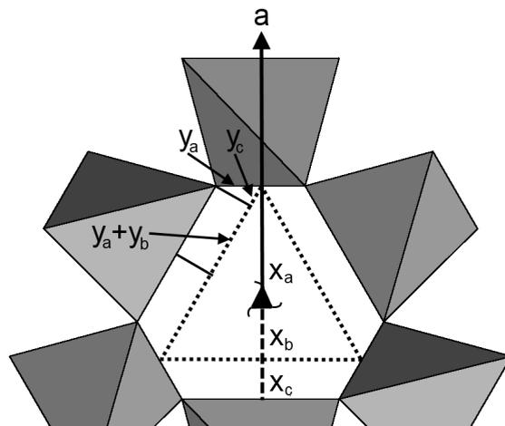
APPENDIX FIGURE 6. Important quantities in deriving  $a$ ,  $x_{O2}$ , and  $y_{O2}$ . This ideal quartz structure in this example has an Si-O-Si angle of  $145^\circ$  and a tetrahedral rotation angle,  $\phi$ , of  $15.4^\circ$ .
