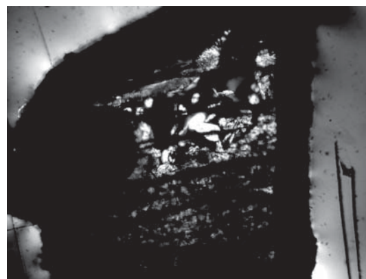
FIGURE 9. Blow-up of experimental charge from run A65 (Fig. 8) under cross-polarized light, which shows crystals, along with glass, at the top of the capsule. The Pt capsule is approximately 3.90 mm from top to bottom.
