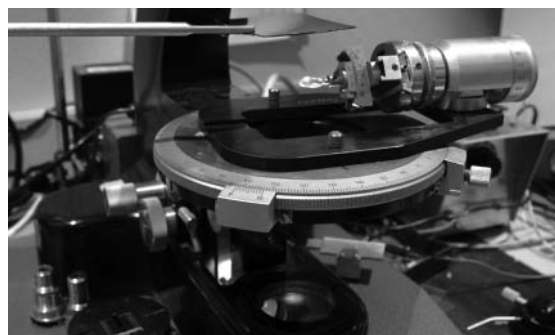
FIGURE 3. The set up used to collect extinction data in air for centimeter-sized single crystals. The objective and substage systems have been removed from the microscope, and sheet polarizers were placed above and below the sample with the vibration directions crossed. Next, extinction positions are observed at the differing S settings (as is typical for use of EXCALIBR) by looking straight down on the sample with the naked eye.
