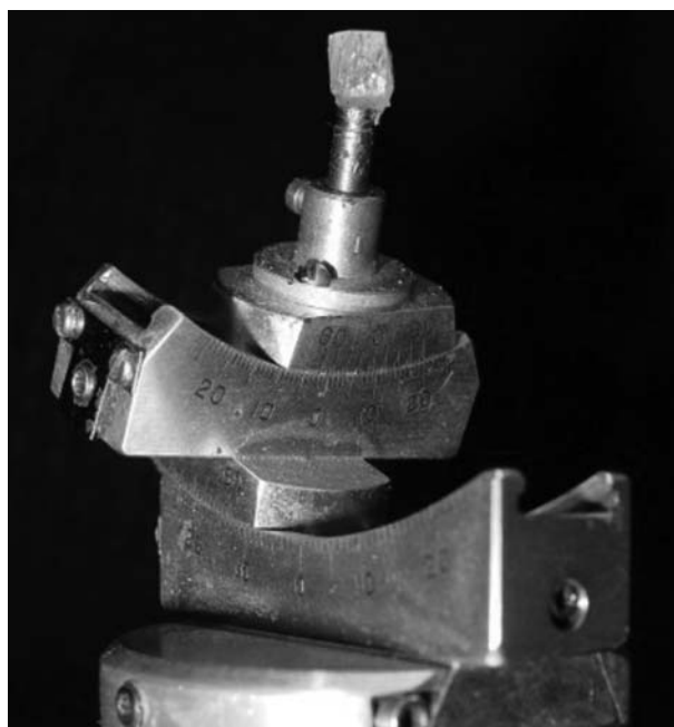
FIGURE 7. A photograph of the spodumene crystal mounted with epoxy on the end of a goniometer head. Notice the size and angular nature of this sample. EXCALIBRW results for this sample are given in Table 4 and Figure 8.
