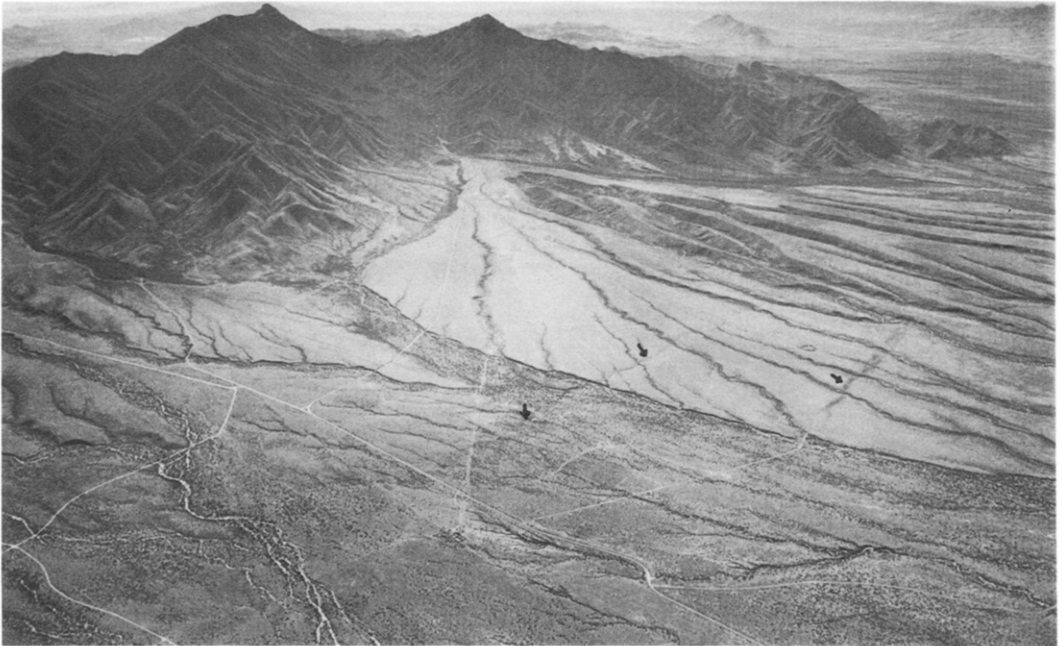
FIG. 2. Aerial view of the Madera Canyon area from the north. Arrows highlight fault scarps that occur on the relatively smooth, light-colored mid-Pleistocene element of Madera Canyon fan (Q2b-1) and slightly darker, late Pleistocene (Q2a) surface to the north. The early Pleistocene element of Madera Canyon fan (Q2a), characterized by much deeper dissection and darker color, is visible south of Q2b-1. The easternmost arrow points to the location of the trench excavated across the fault zone. (Photo courtesy of Peter L. Kresan.)
